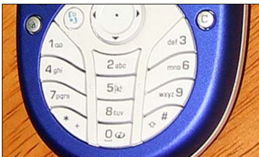
Figure 13 U-shape keypad in Nokia 3660
