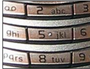
Figure 15 Tactile cue on the 5-key
