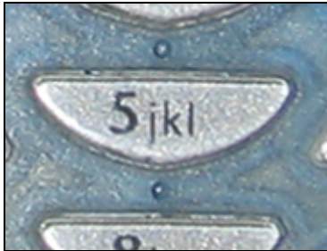
Figure 14 Tactile cue beside the 5-key
