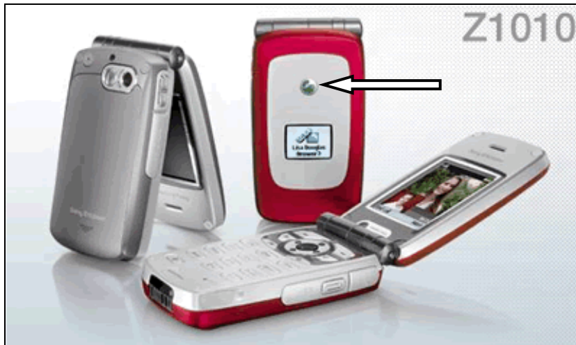
Figure 20 SonyEricsson Z1010 mobile phone (pointing to camera used in one-way video messages)
